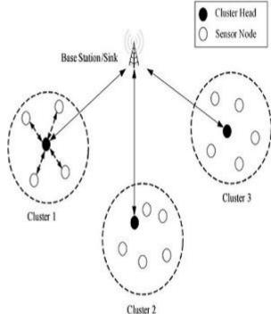
Figure1: Clustering In Wireless Sensor Network
