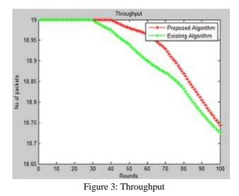
**Throughput due to Existing Algorithm: 14776.28 bps Throughput due to Proposed Algorithm: 15254.02 bps** After the detection and prevention of the network from misdirection attack by removing the malicious node from the network, the packet loss is reduced greatly depicted by the red colored marks in the figure 4.
