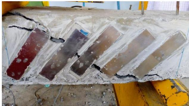
Fig.7 Failure mode of AA45 beam
