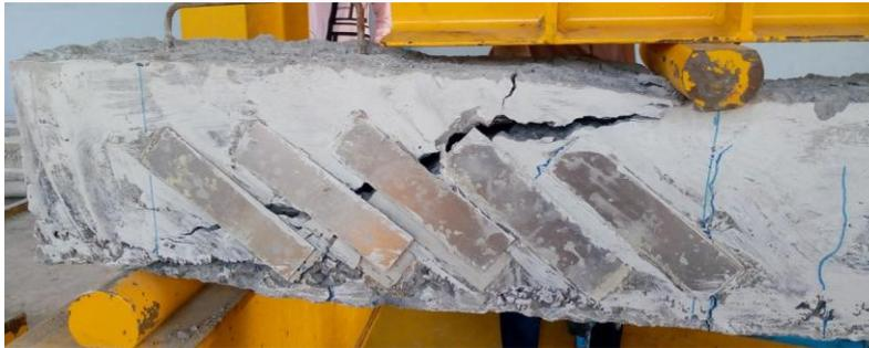
Fig.6 Failure mode of AA30 beam
