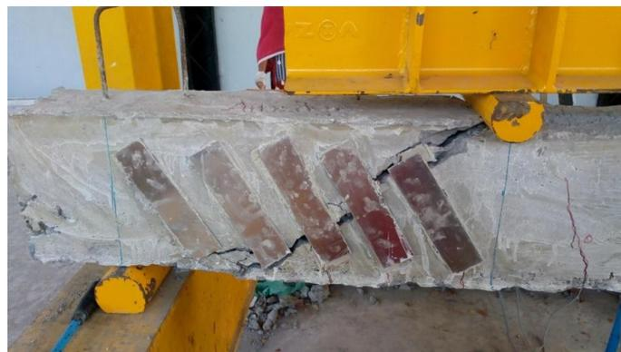
Fig.8 Failure mode of AA60 beam
