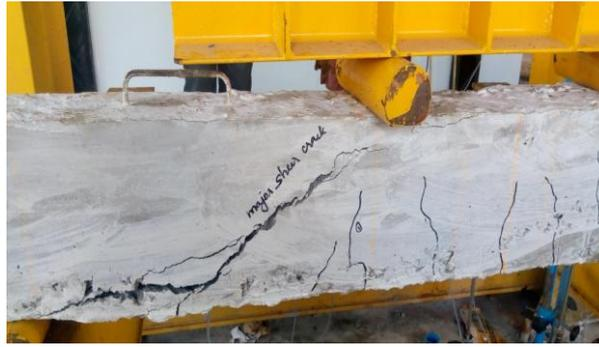
Fig.5 Failure mode of Control beam
