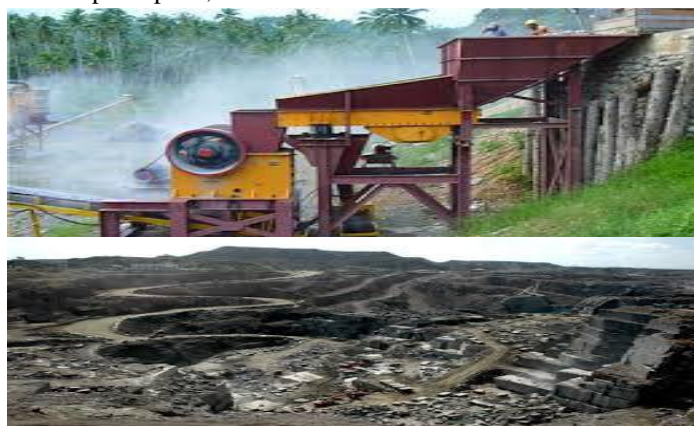
Fig no: 02 Production of Quarry Dust in a Crushing Plant
