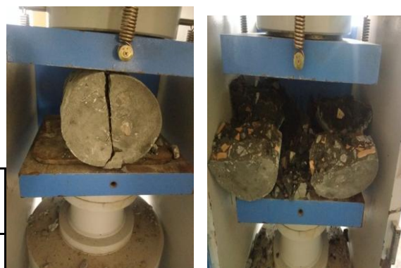
Fig 4.3: Split Tensile Testing and Specimen (Cylinders)
