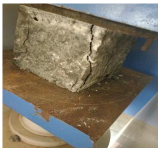
Fig 4.1: Compression testing of Cube Specimen
