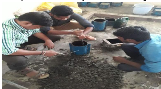
Fig 3.2: Hand mixing and placing of concrete mix
