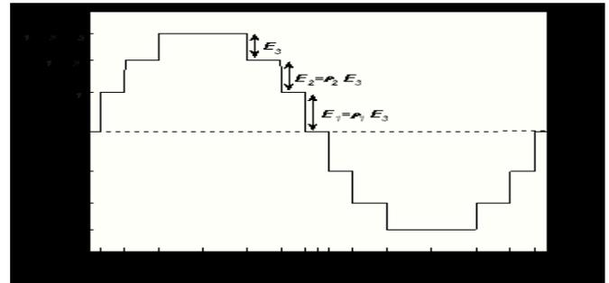
Fig. 3.2 A 3-step (7-level) waveform defined by its step angle and voltage ratio parameters.
