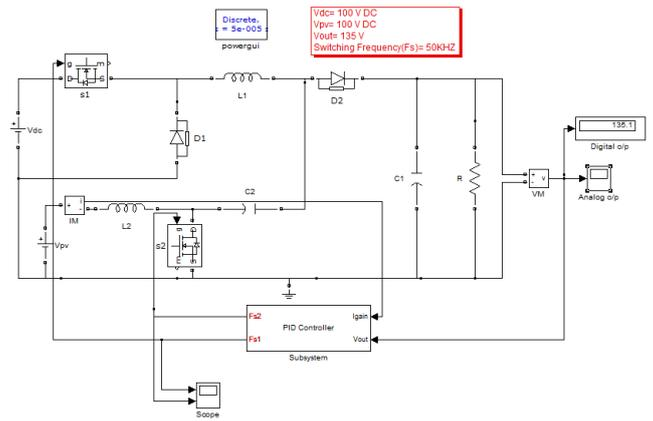
Simulink model for closed loop control of Buck-integrated SEPIC converter
