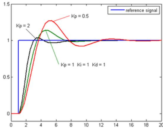
**Plot of PV vs time, for three values of  $K_p$  ( $K_i$  and  $K_d$  held constant)**
