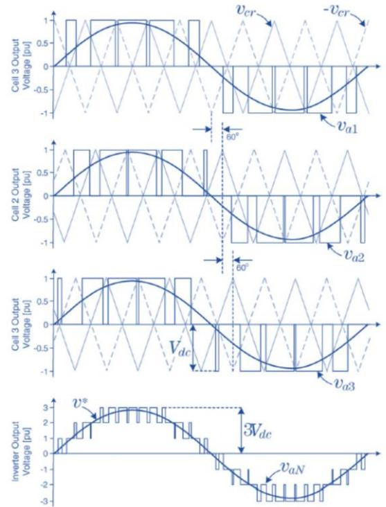
Three cell PS-PWM waveform generation
