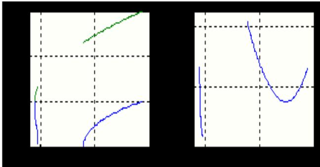
Minimum WTHD, and Fig3.5 (b) corresponding optimal  $\rho_1$  versus  $m_1$ ; harmonic eliminating case.
