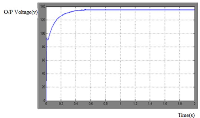
Simulation result for closed loop control of Buck-integrated SEPIC converter
