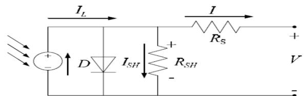
**Equivalent Circuit of a PV Cell**
