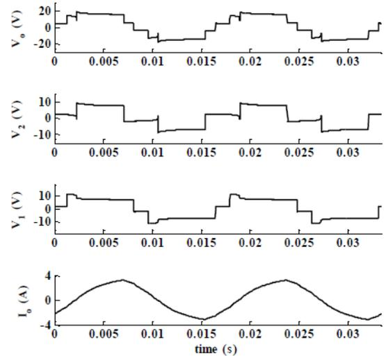
Fig. 13. Output voltage (5-level) of the inverter for optimal THD with a 0.8 lagging pf load and 20%Vswd.
