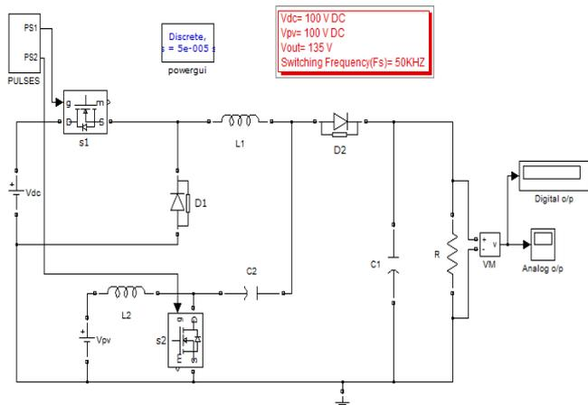
Simulink model for open loop control of Buck-integrated SEPIC converter
