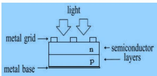
**Structure of a PV Cell**
