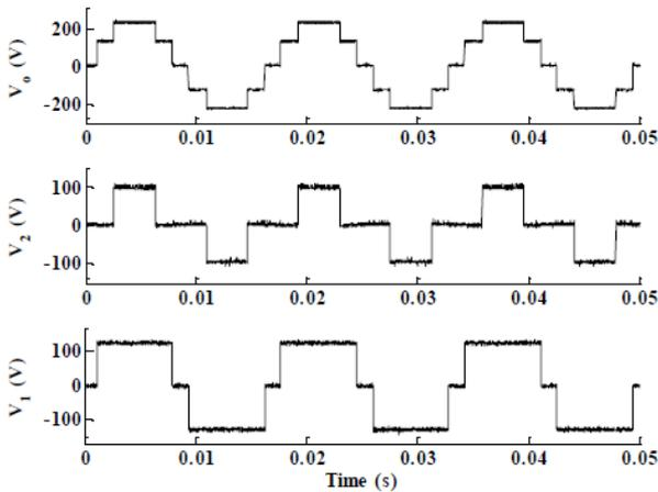
Fig. 5.8 Output voltage (5-level) of the inverter and output voltage of each H-bridge to achieve optimal THD with HE.
