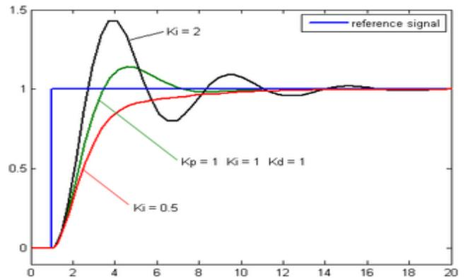
**Fig 4.13 Plot of PV vs time, for three values of  $K_i$  ( $K_p$  and  $K_d$  held constant)**
