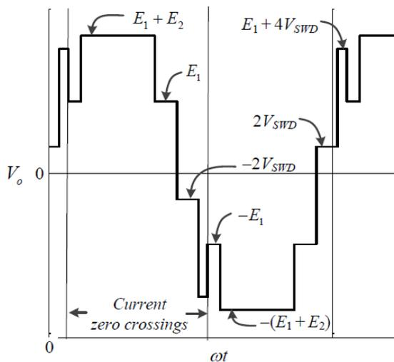
Inverter output voltage (5-level) waveform considering device voltage drops for a moderately-lagging power factor load.
