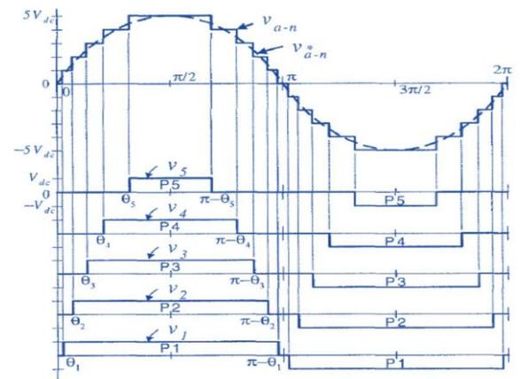
Output waveform of a 9-level cascade inverter
