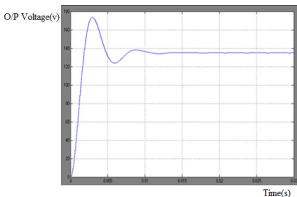
Simulation result for open loop control of Buck-integrated SEPIC converter
