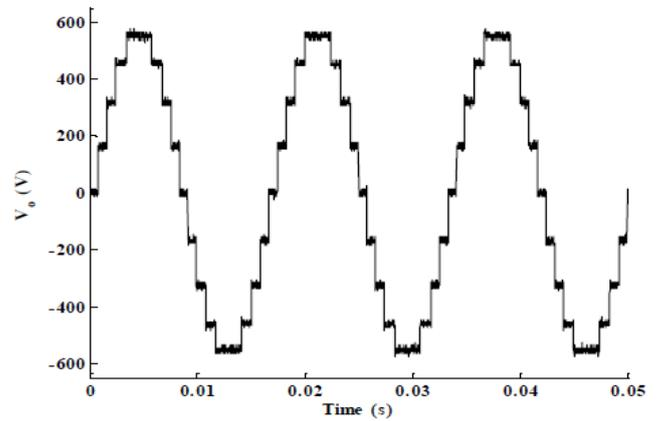
Fig.5.10. Output voltage (9-level) of the inverter for optimal THD.
