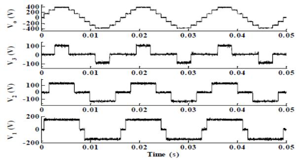
Output voltage (7-level) of the inverter and output voltage of each H-bridge to achieve optimal WTHD.
