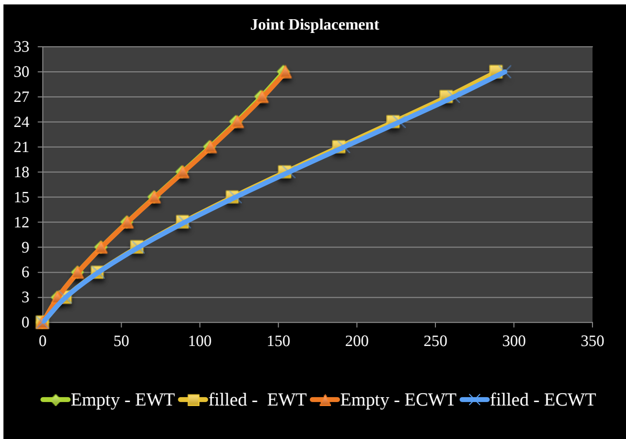
Fig. 6: Joint Displacement Due to Load Combination 1.2 (DL+EQL+WP)
