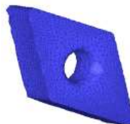
Figure 3: WIDIA CNMG 120408 in Deform 3D
