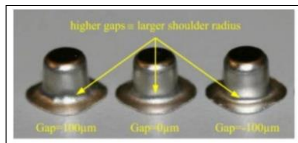
Figure 4. Cups formed with different initial gaps [12]
