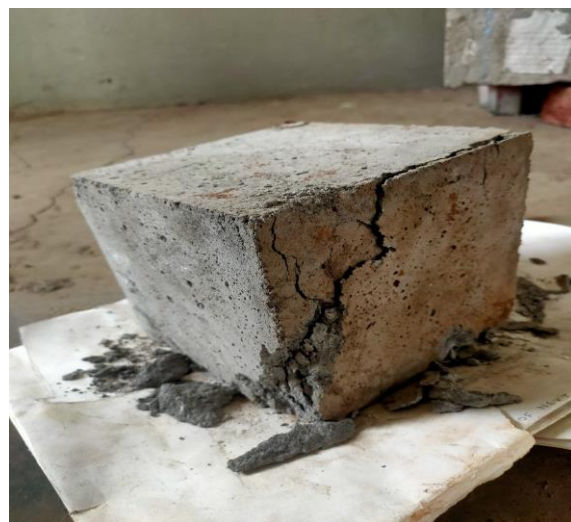
Fig. 5 Failure Pattern after 28 days on cube. (sample 2)
