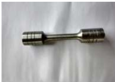
Figure 5.6 Specimen before Tensile test
