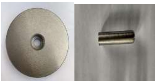
Figure 5.11 Specimen before Wear test
