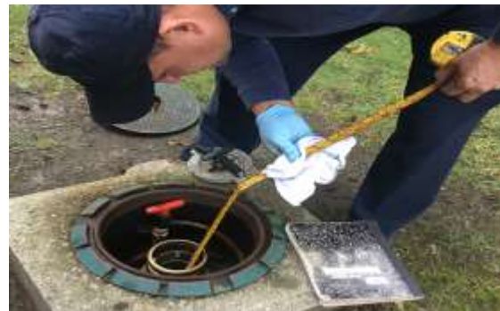
Fig 1: A Technician taking fuel measurement in underground tank with Measuring tape [6]
