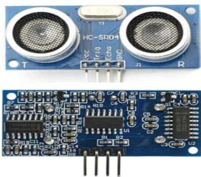
Fig 3: Ultrasonic range finder module [11]
