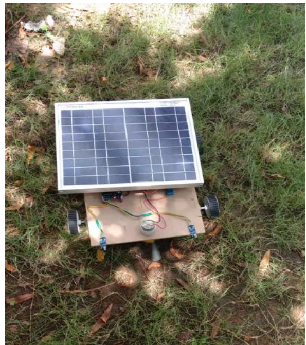
Fig.1.4. Hardware implementation Of The Proposed System
