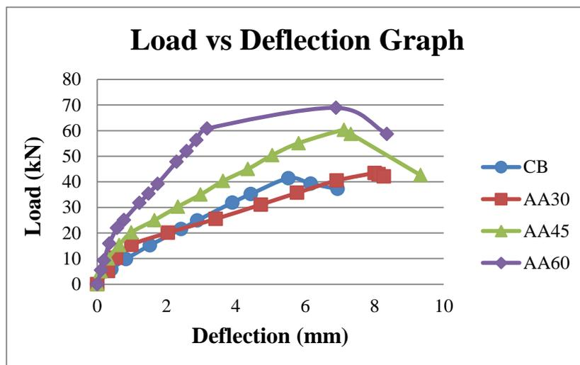
Fig.4 Load- deflection curves for all tested beams
