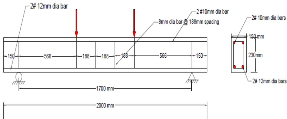
Fig. 1 Reinforcement profile and cross section
