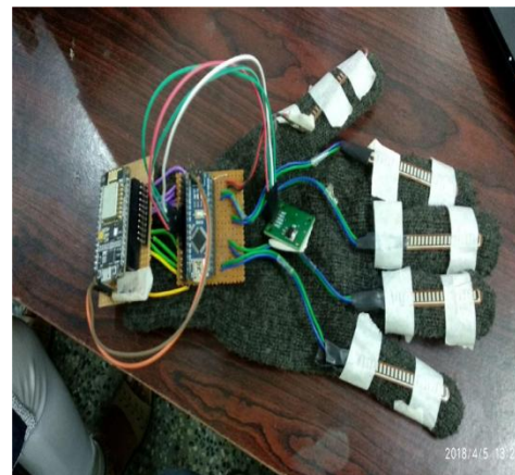
Fig.10:Shows Controlling the Wheel Chair with Hand Gestures
