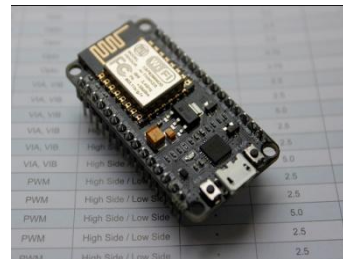
Fig: 2 NODE MCU board
