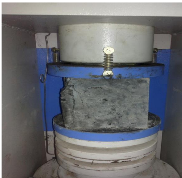
Figure 7.1 Showing Compressive testing of cube with Compression testing Machine
