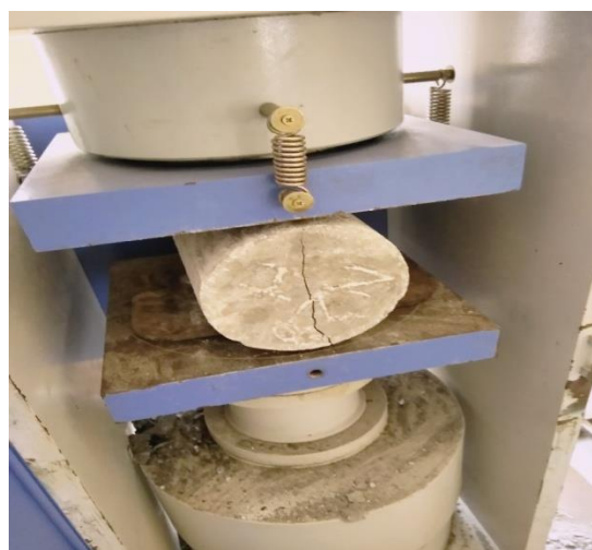
Figure 7.2 Showing Split Tensile testing of cylinder with Compression testing Machine
