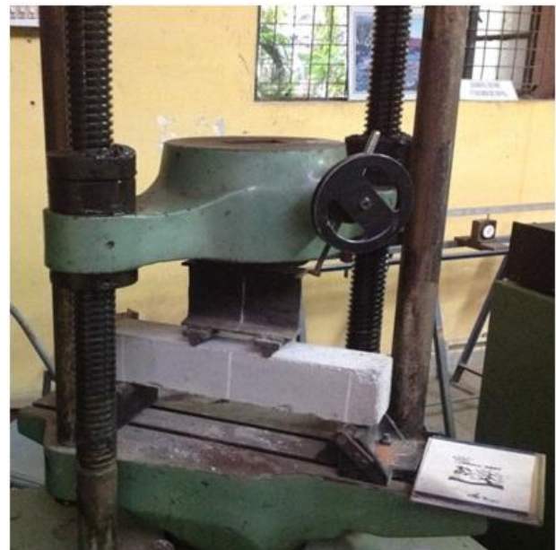
Experimental Setup for Flexure Test
