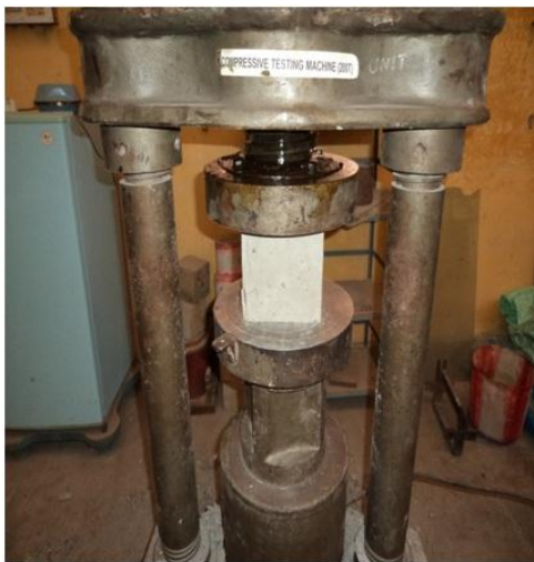
Fig 4.1: Compression testing of Cube Specimen
