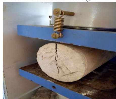
Figure 6 Split tube tensile test apparatus
