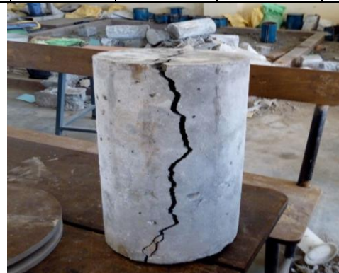
Figure 13 Split tensile Strength test of concrete cylinders
