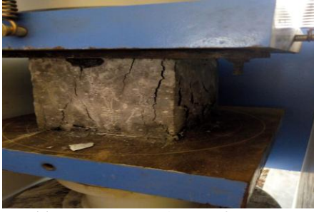
Figure 11 Comp. Strength test of concrete cubes
