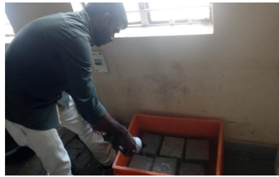
Figure 16 Placing of concrete cubes in acid curing.
