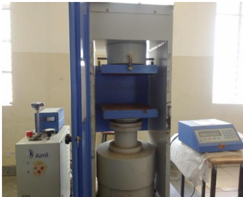
Figure 5 Compression testing machine
