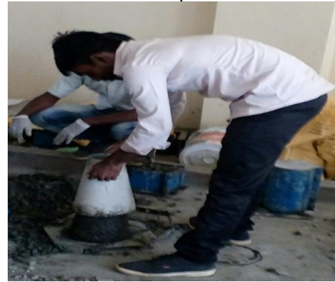
Figure 9 Slump cone test
