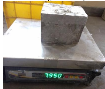
Figure 17 Weighing of concrete cube after 28 days acid curing.
