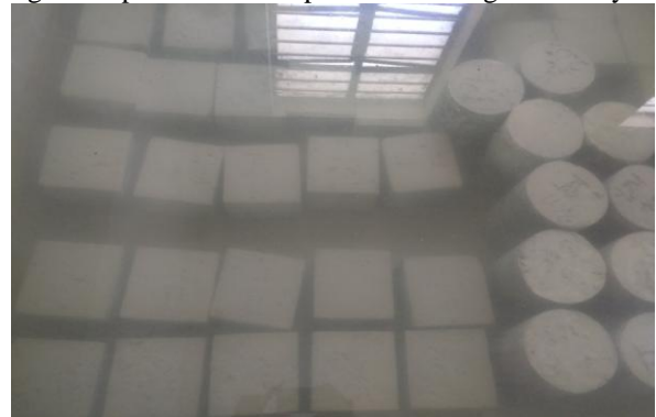
Figure 3. Curing of concrete cubes & cylinders.
