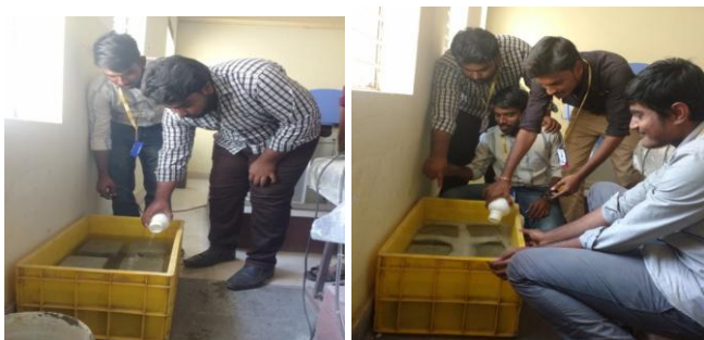
Figure 19 placing of concrete cubes in alkali curing.
