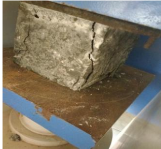
Fig 4.1: Compression testing of Cube Specimen
