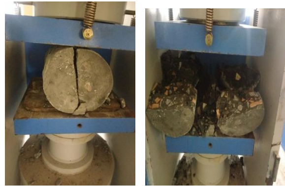
Fig 4.3: Split Tensile Testing and Specimen (Cylinders)
