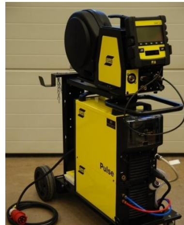
Fig.1 Pulse GMAW machine ESAB Aristo MIG 4004I used in the experiment
