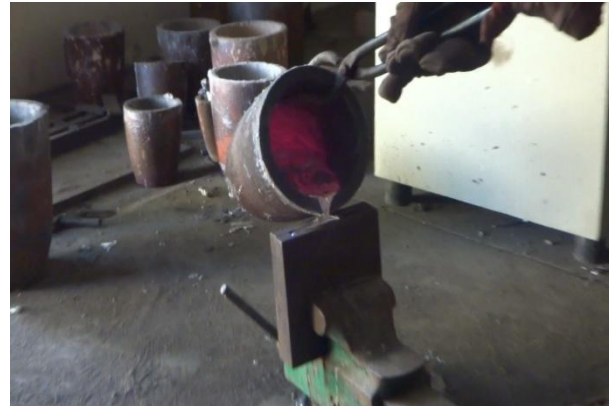
Fig.3 Gravity die casting of liquid MMC
