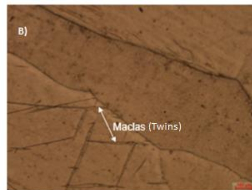
Fig 3: Microstructures of commercially pure magnesium in the "as received" (a) and pre-homogenized (b).
