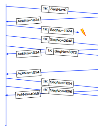
Fig.3.1.2. Sequence diagram for Fast Recovery
