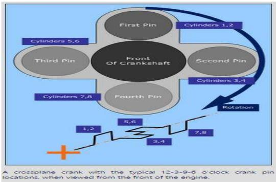
Fig 3 Cross plane type of V8 Engine
