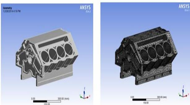
Fig 10 Geometry & Meshing of Cylinder Block
