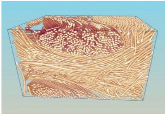
Fig 6 Carbon Fibre Reinforced Carbon
