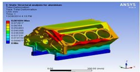
Fig 14 Total deformation generated in cylinder block
