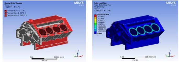
Fig 11 Steady state & Total Heat Flux
