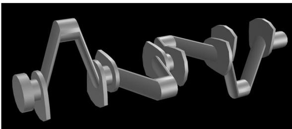
Fig 4 Cross Plane crankshaft
