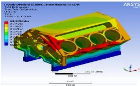
The above Fig 16 shows the total deformation induced in the cylinder block for FU 4270 material.
