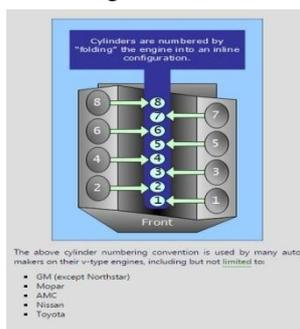
Fig 1.1 No of cylinders showing in V8 Engine
