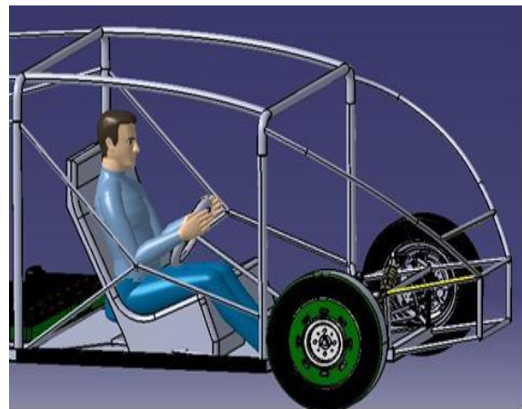
Fig. 1. Ergonomic setup designed in CATIA.
