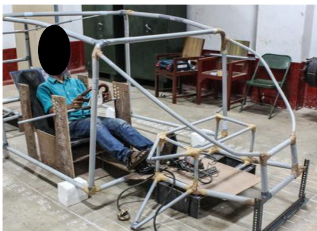
Fig. 5. PVC chassis with ergonomic apparatus.
