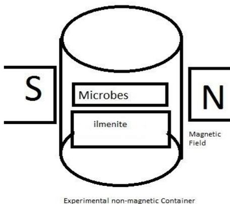
Fig. 1 Experimental arrangement for synthesis of ilmenite nanoparticles
