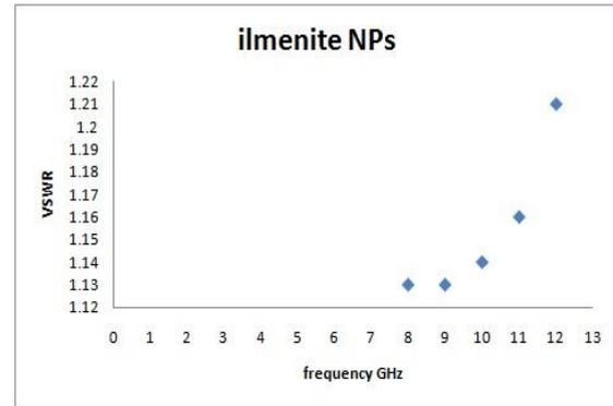
Fig. 4 Graph plotted between VSWR and Frequency.
