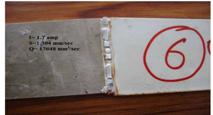
Figure 7 Weld bead formed in 6 th experiment
