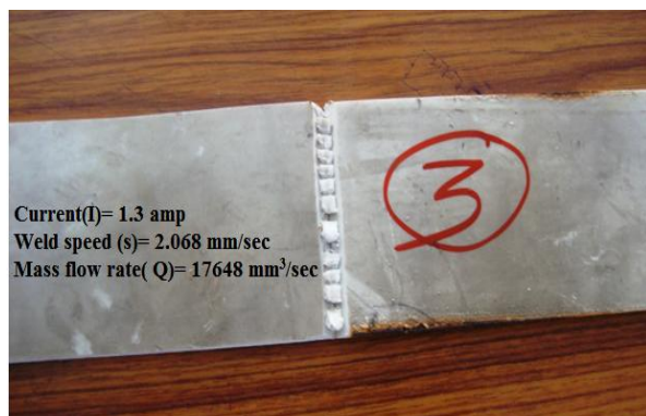
Figure 4 Weld bead formed in 3 rd experiment
